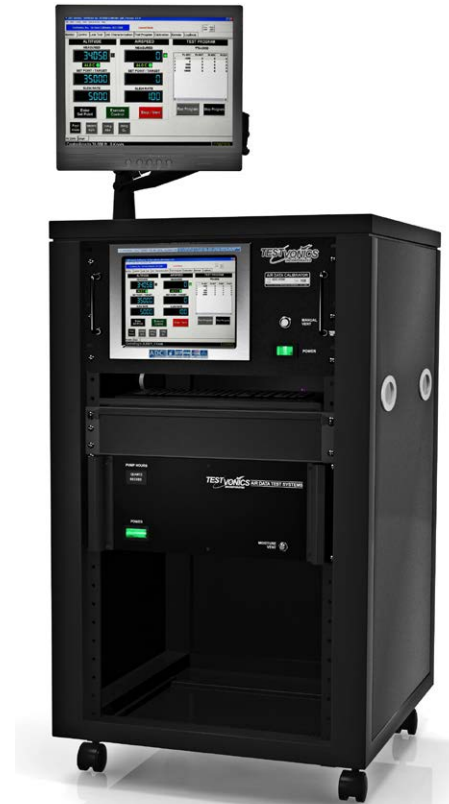
(above) ADTS-1555 Series Calibrator with Vacuum Pressure unit, External Touchscreen Monitor and Rackmount Enclosure
